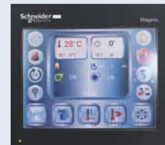
Touch screen con PLC. Touch screen control panel with PLC.
