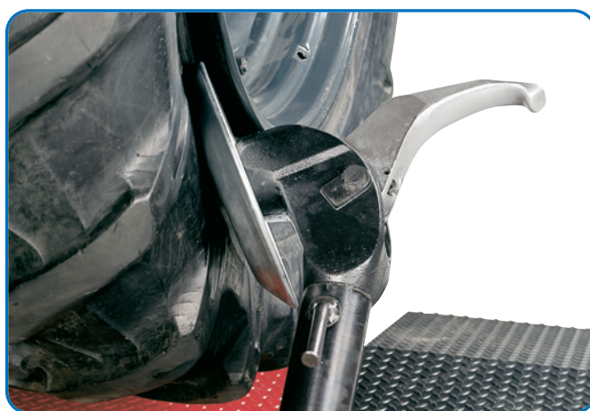
➤ Pneumatic bead breaking
