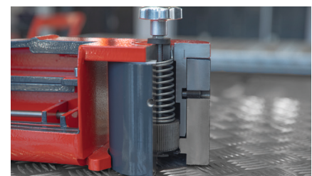
Internal arm locking system
