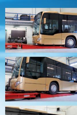
In doing so, vehicle configurations of up to 30 metres in length and with a total weight of up to 70 tonnes can easily be lifted! The SKYLIFT is even flexible with regard to its width. During installation, the width between the platforms can be adjusted to the fleet of vehicles.
